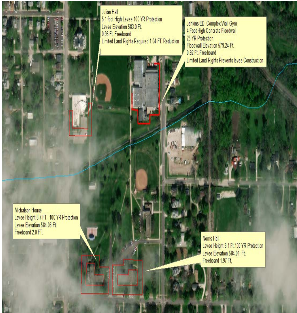
Figure 22 - Alternative 7 – Plan View of Floodproofed MacMurray Structures
